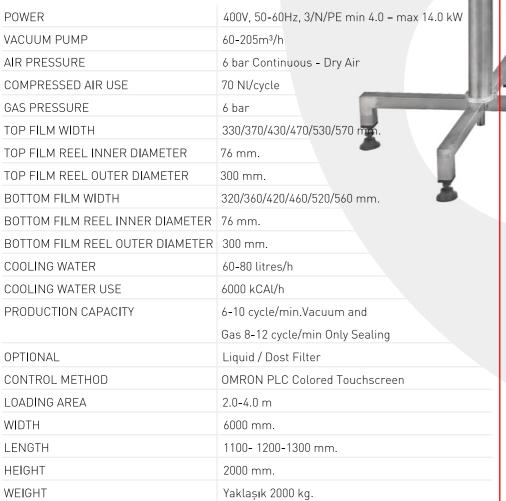
The entire body of our machines is made of stainless steel. Belt conveyors and moving parts are made of hygienic materials. The machine is very easy to use, maintain, and clean.
