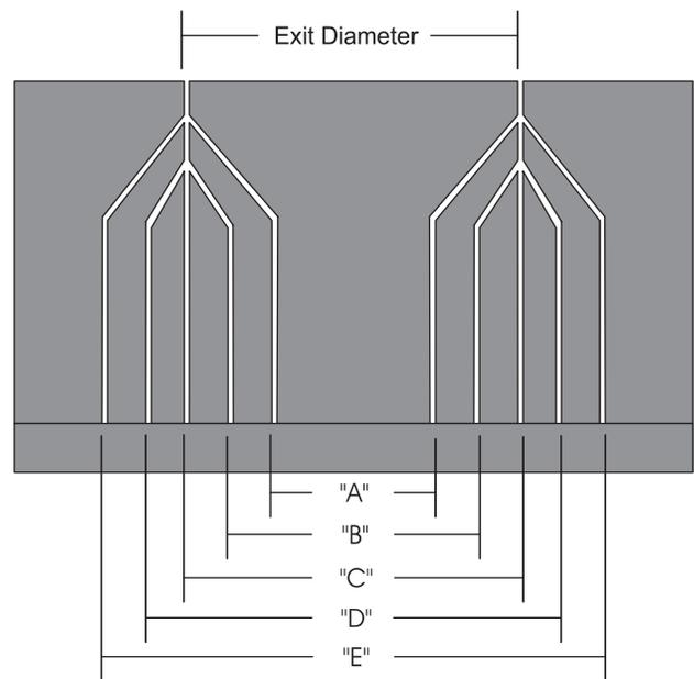
Fig. 7-2 Conventional coextrusion die consisting of five nested cylinders.
