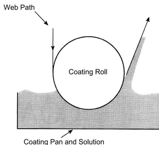
**Fig. 13-5** Dip coater. From Modern Coating and Drying Technology, (Cohen, E.D., Gutoff, E.B., eds), Copyright © 1992 Wiley-VCH. Reprinted with permission of John Wiley & Sons, Inc.
