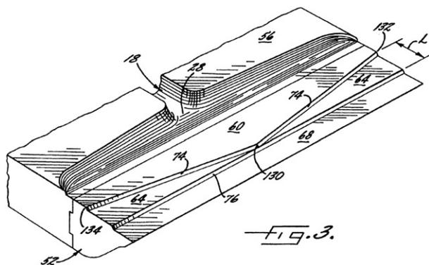
**Fig. 6-24** Cloeren Inc. inverted preland die design (Figure 3 of US Patent 5,256,052) showing initial damming land (60) followed by deeper lands 64 and 68. The transition from 60 to 64 is a function of position across the die width and is dependent on the melt rheology.
