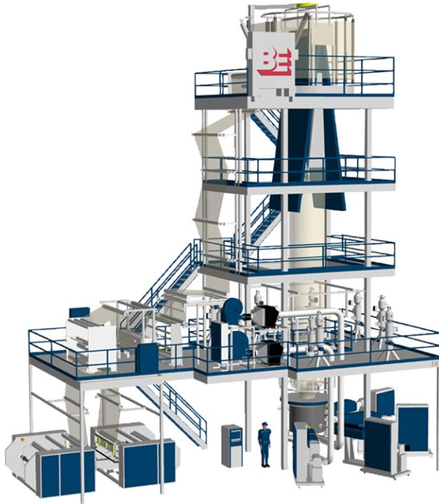
**Fig. 9-2** Seven-layer blown film 3D layout. Image provided by BE (Brampton Engineering) [www.be-ca.com](http://www.be-ca.com).
