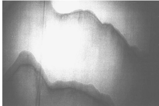
Fig. 7-10 Two-layer tubular film with interfacial instability.
