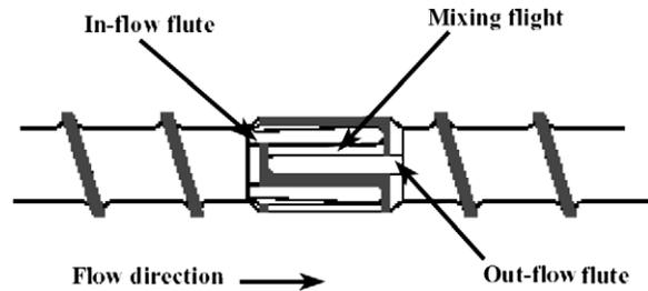
**Fig. 12-7** Maddock screw element (adopted from Spalding and Hyun [20]). Courtesy of the Society of Plastics Engineers.
