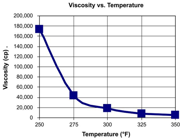
**Fig. 13-17** Viscosity–temperature relationship for a hot melt coater.
