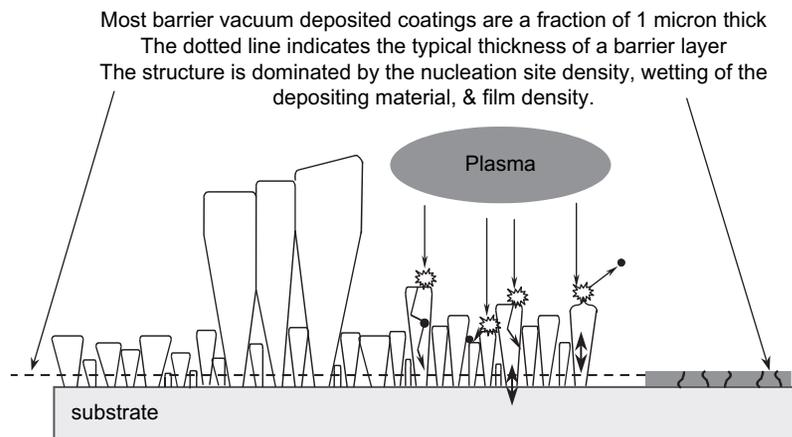
**Fig. 14-19** A schematic of the nucleation and growth of a thin film coating.
