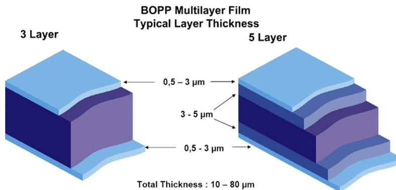
Fig. 16-6 Typical layer thickness of BOPP multilayer film.
