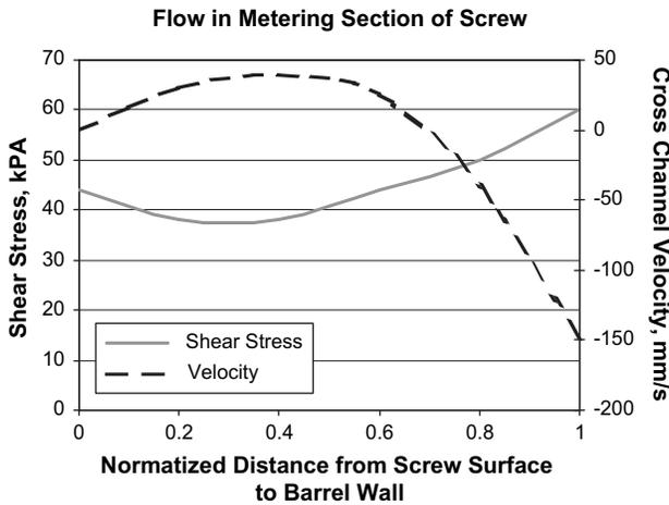
**Fig. 12-4** Example of stress and velocity distribution of polyethylene in the cross channel direction of the metering section of a single-screw extruder. Calculations were done using commercial software from Polydynamics, Inc.
