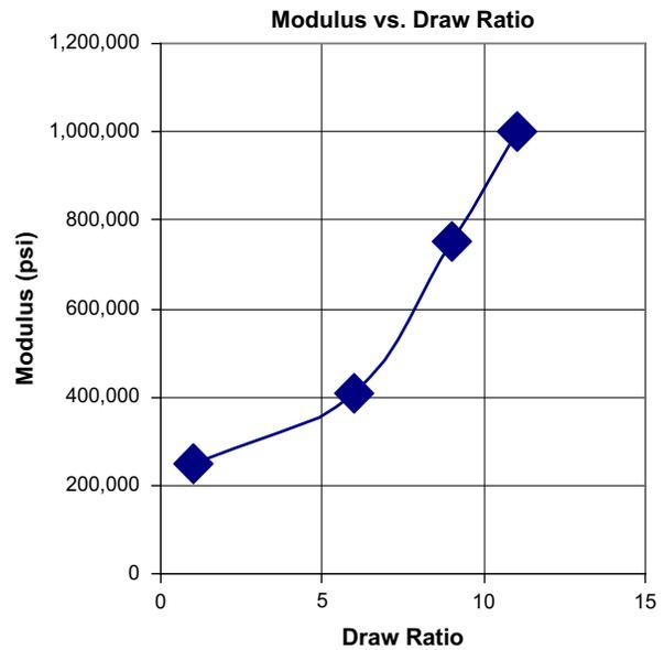
**Fig. 10-11** MD modulus versus draw ratio for HMW HDPE [4].
