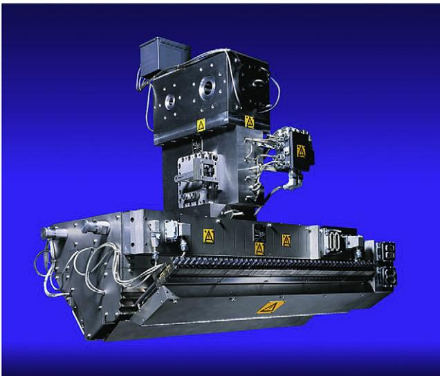
**Fig. 6-1** General configuration the coextrusion system consisting of an adapter, a feedblock and a single or multicavity die (courtesy Cloeren Company).
