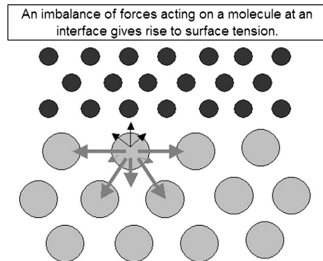
**Fig. 12-14** Illustration of the origins of interfacial tension.
