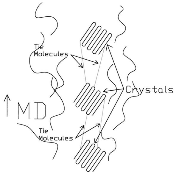
**Fig. 10-4** Continued tie molecule orientation as the polymer is stretched further.
