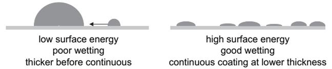
**Fig. 14-18** A schematic diagram showing how surface energy can affect the wetting and hence coating quality.
