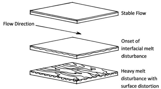
**Fig. 6-30** Schematic diagram of two-layer flow showing the transition from stable to heavy melt disturbance with film distortion.
