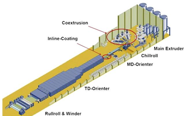
Fig. 16-2 Multilayer structures in Biaxially Orienting Lines.
