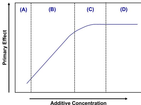
**Fig. 4-3** Concentration dependency of the primary effect of additives.
