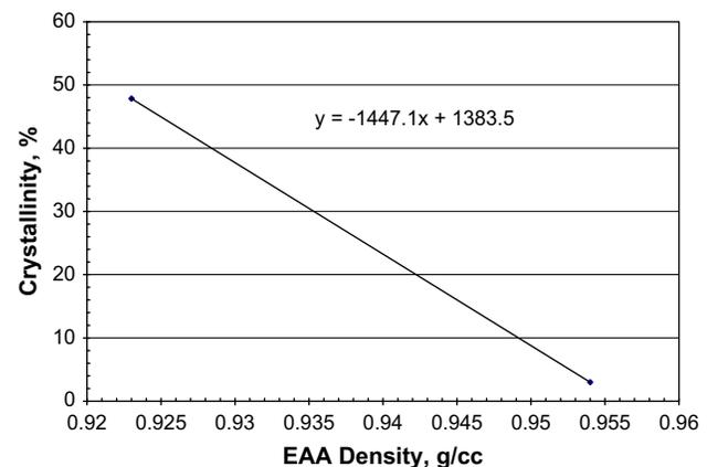
Fig. 2-22 EAA crystallinity as a function of density.
