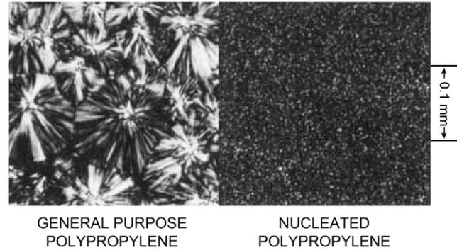
**Fig. 3-6** Two optical micrographs show the effect of a nucleating agent on spherulite size. In nucleated polypropylene, right, spherulites are smaller and more numerous than in un-nucleated polypropylene, left.
