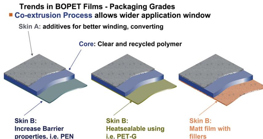
Fig. 11-22 Coextrusion trends in BOPET.
