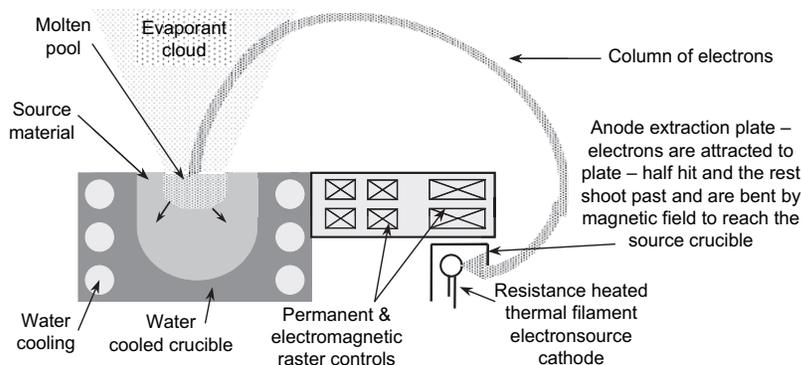
Fig. 14-14 A schematic of a small electron beam gun.
