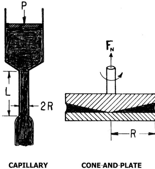
Fig. 5-6 Schematic representation of a capillary and a cone-and-plate viscometer.
