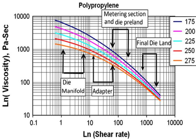
**Fig. 6-11** Shear rate ranges in various locations in multilayer extrusion equipment.
