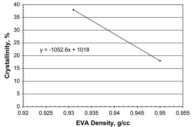
Fig. 2-20 EVA crystallinity as a function of density.
