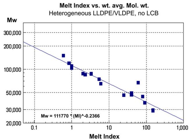
Fig. 2-5 Melt index as a function of  $M_w$ .
