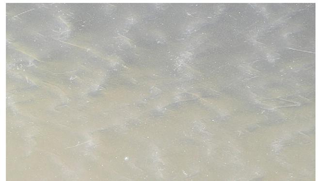
**Fig. 6-27** Melt disturbance of a three-layer sheet showing distortion of the sheet and the chevron appearance of the flow.
