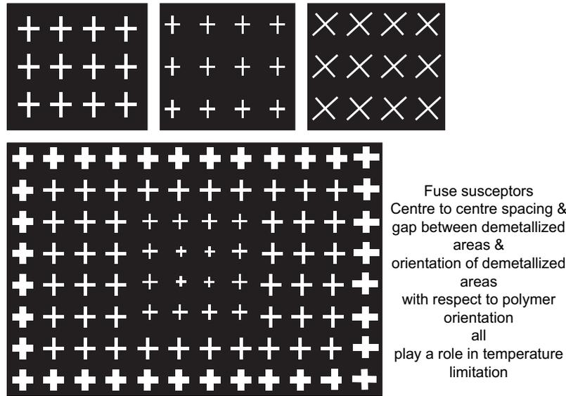
Fig. 14-8 Various fused susceptor designs. The white areas are demetallized.
