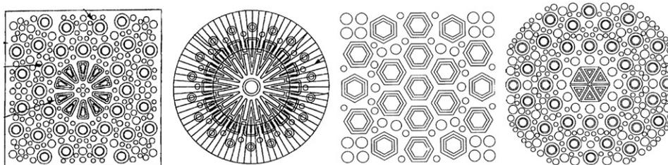
Fig. 14-7 A variety of patterns produced for microwave heating of foods [20].
