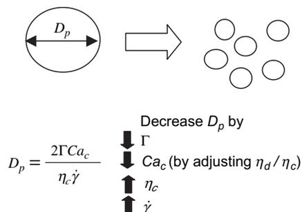
Fig. 12-17 Learnings from single droplet mechanics.
