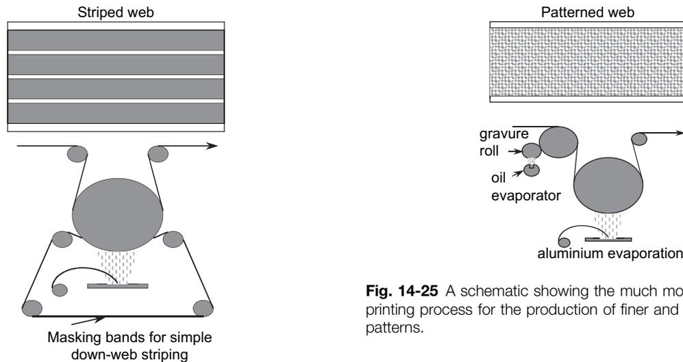
**Fig. 14-24** A schematic showing the process of using a masking band that produces simple stripes.
