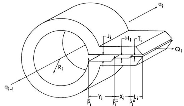
**Fig. 6-21** Schematic diagram of die with a straight tapered circular manifold and a three gap die land where the three land lengths were a function of position across the die width (Redrawn from [6]).
