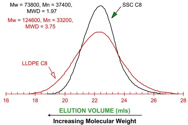
**Fig. 2-39** MWD comparison between Z-N LLDPE and SSC octene copolymers of similar MI and density (1.0 MI, 0.920 g/cc).
