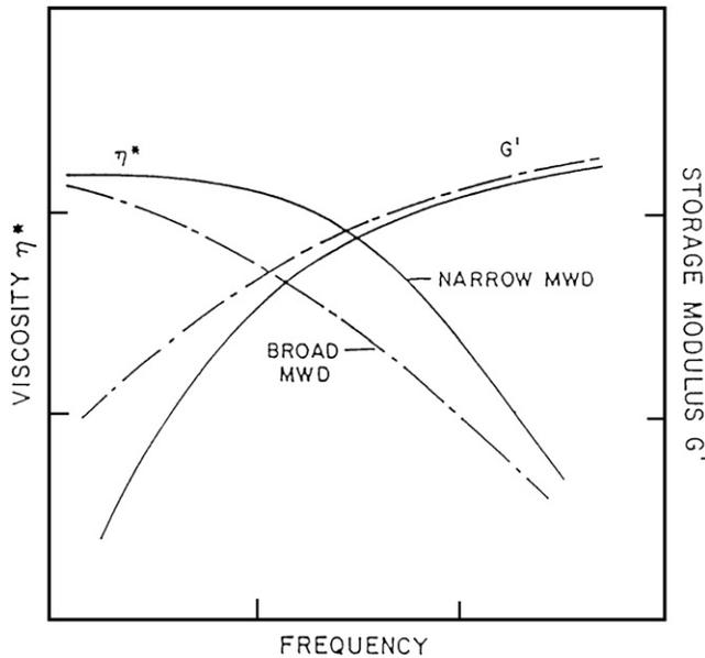
**Fig. 5-11** Storage modulus  $G'$  and dynamic viscosity  $\eta^*$  behavior of broad and narrow molecular weight distribution polymers.
