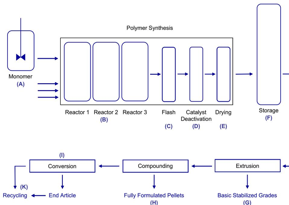
Fig. 4-1 Addition points for additives during the life time of a substrate (modified from [1]).
