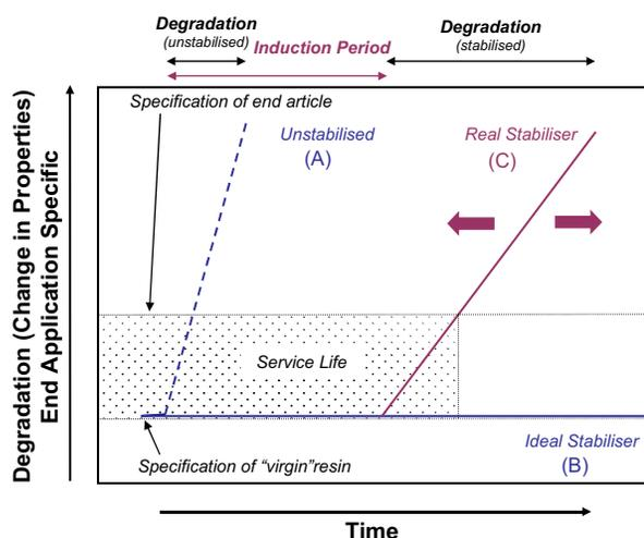
Fig. 4-5 Principle for the utilization of antioxidants (and other stabilizers) during service life (modified and improved from [5]).
