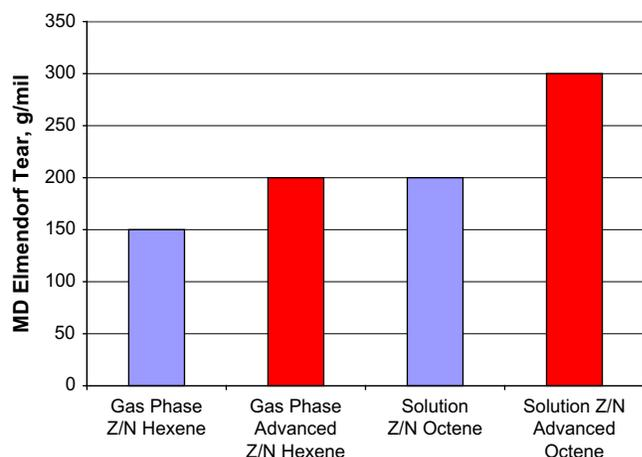
**Fig. 2-35** Comparison of different Z–N catalyst systems in both gas phase and solution process on MD Elmendorf tear strength.
