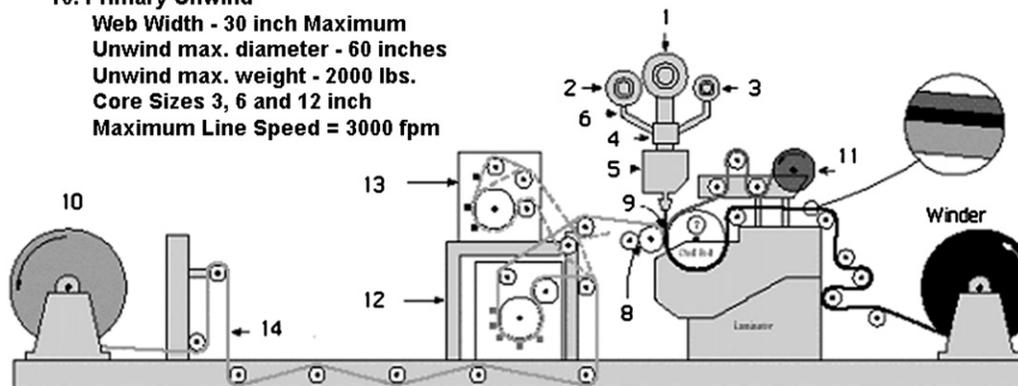
**Fig. 9-10** High speed laboratory extrusion lamination line.
