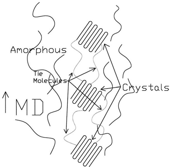
**Fig. 10-3** Initial tie molecule orientation as the polymer starts to be stretched.
