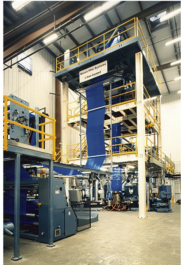
**Fig. 9-4** Blown film tower and collapsed film going to winder. Image provided by Davis-Standard <http://www.davis-standard.com/>.
