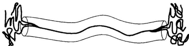
Fig. 5-13 The Pom-Pom polymer model.
