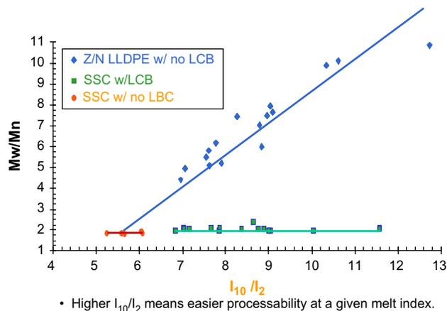
Fig. 2-41 Comparison of LLDPE, m-LLDPE and SSC w/LCB on the relationship of MWD and  $I_{10}/I_2$ .
