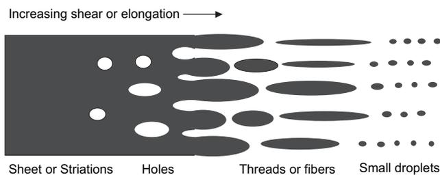
**Fig. 12-24** Morphology development during melting and subsequent shear in an extruder. Striations or sheets form during melting. Shear and stress cause holes to form, followed by threads and particle break-up. This process leads to large changes in the minor phase morphology.
