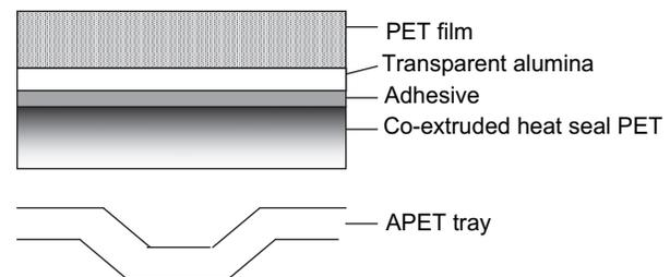
**Fig. 14-29** PET heat-seal laminate barrier-lidding material.
