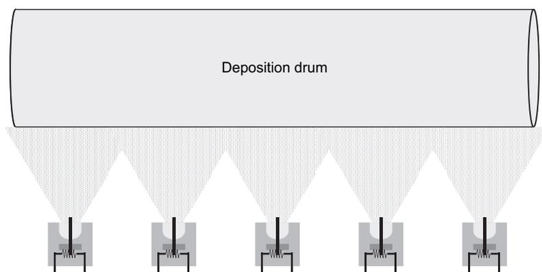
Fig. 14-15 A schematic of a series of electron beam deposition sources showing them arranged for overlapping deposition.
