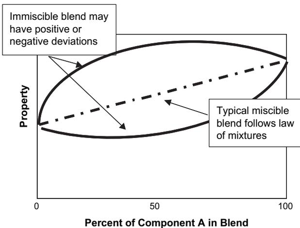
**Fig. 12-11** Properties versus percent A in polymer blends.
