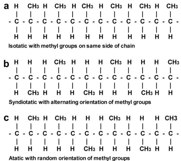
**Fig. 3-2** A schematic of polypropylene tacticities: (a) isotactic with all methyl groups on the same side of the chain; (b) syndiotactic with methyl groups alternating above and below the chain; (c) atactic with methyl groups in a random orientation.
