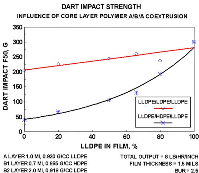
Fig. 15-1 Influence of polymer in core layer.
