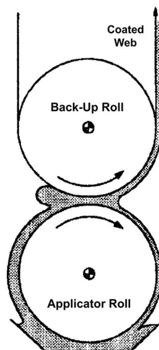
**Fig. 13-6** Two-roll, pan fed forward roll coater. From *Modern Coating and Drying Technology*, (Cohen, E.D., Gutoff, E.B., eds), Copyright © 1992 Wiley-VCH. Reprinted with permission of John Wiley & Sons, Inc.
