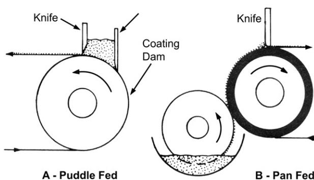
**Fig. 13-10** Knife-over-roll coater. From H. Weiss, *Coating and Laminating Machines*, Converting Technology Co., Milwaukee, 1977, with permission of Mrs Sheila Weiss.
