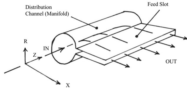
**Fig. 6-20** Schematic diagram of end feed die showing flow into and through the manifold and die land.
