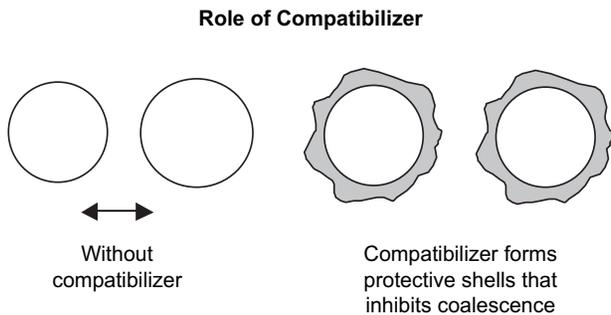
Fig. 12-19 Role of compatibilizers in reducing coalescence in polymer blends.
