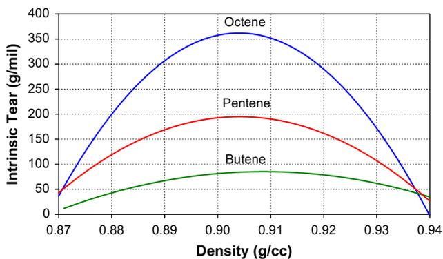
**Fig. 2-44** Intrinsic tear as a function of density for octene, pentene and butene copolymers.
