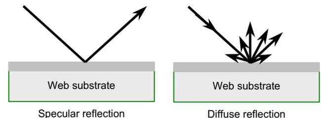
Fig. 14-3 A schematic diagram showing the difference between specular and diffuse reflective coatings.
