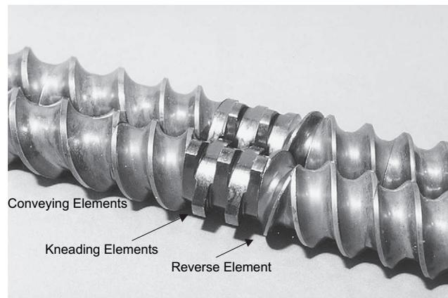
Fig. 12-9 Twin-screw extruder modular elements.
