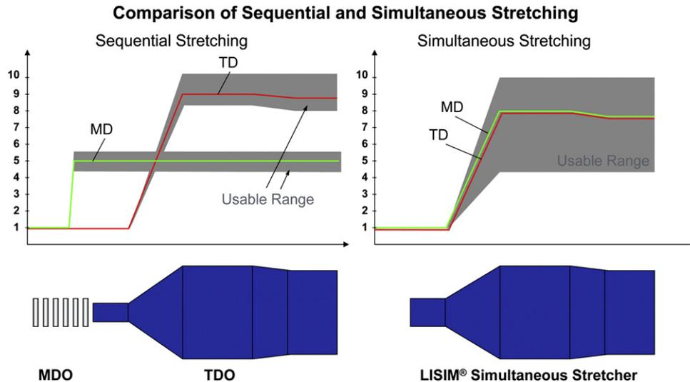
**Fig. 11-10** Useable stretch ratios for sequential and simultaneous stretching.
