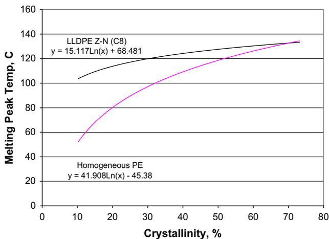
Fig. 2-33 Peak melting temperature for homogeneous PE versus crystallinity is compared to heterogeneous LLDPE octene copolymers from a solution process.
