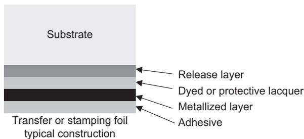
Fig. 14-2 Schematic of hot or cold stamping foil: foil construction.
