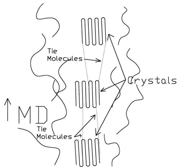
**Fig. 10-5** Fully stretched tie molecules rotate crystals to bring them into alignment.
