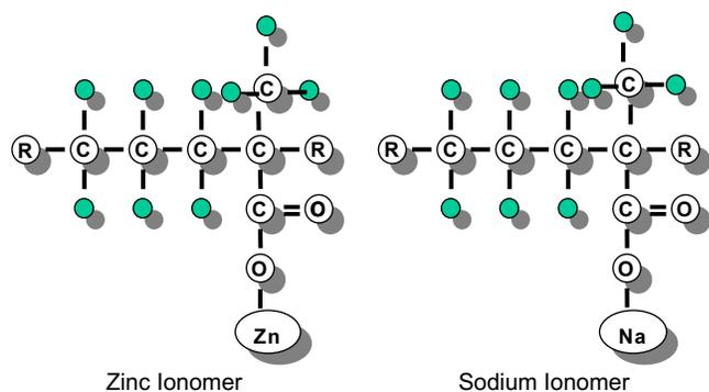
Fig. 2-23 Zinc and sodium ionomers.
