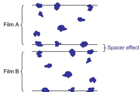
Fig. 4-7 Principal mode of action of inert, inorganic antiblock additives.
