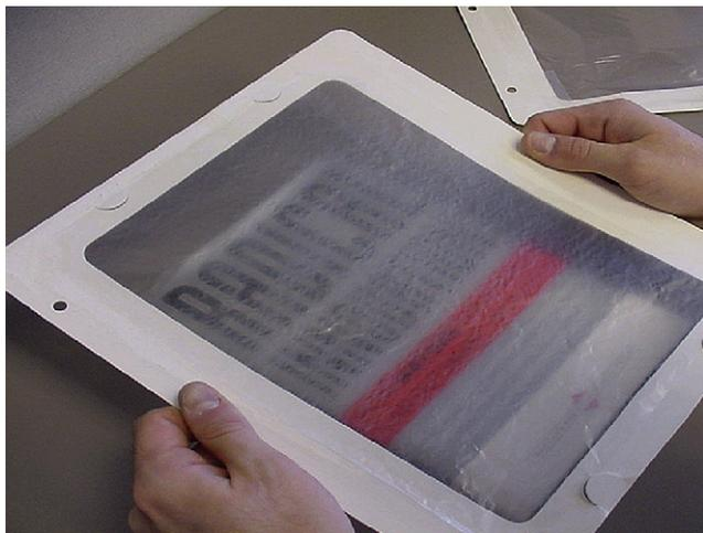
Fig. 10-7 Poor see through clarity of un-oriented film [2].
