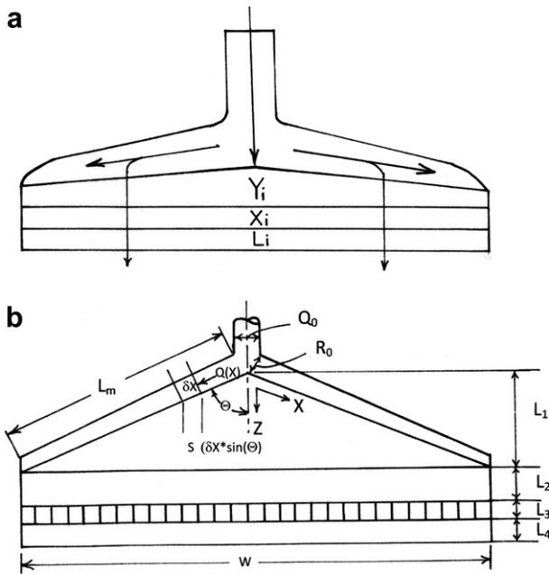
**Fig. 6-22**(a) Coat hanger die with three variable depth lands ( $Y_i, X_i, L_i$ ) as in [6]; (b) coat hanger die of Chung and Lohkamp (redrawn from [8]).
