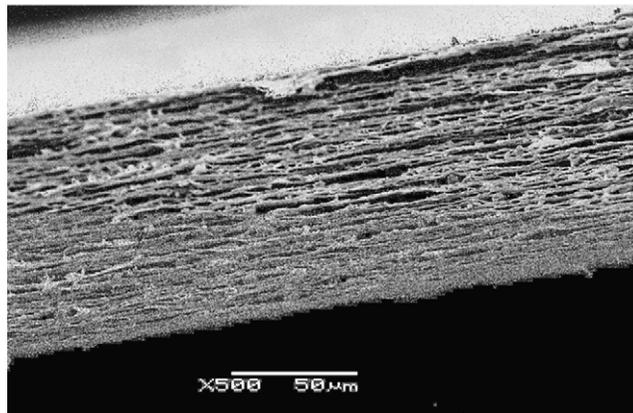
Fig. 11-18 Cross-section of 100 µm BOPP synthetic paper showing the calcium carbonate particles, cavities and uncavitated skin layers.
