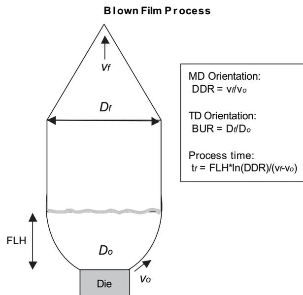
Fig. 12-26 Blown film process.
