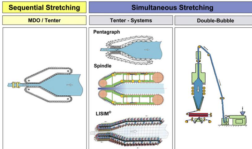
Fig. 11-5 Biaxial orientation.
