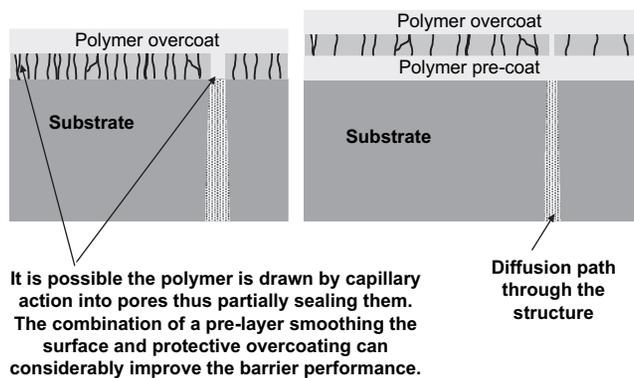
**Fig. 14-22** A schematic showing the benefits of minimizing surface defects.
