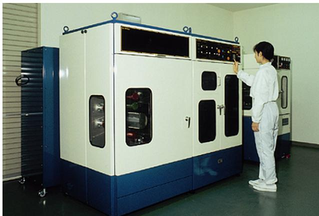
**Fig. 13-2** Yasui Seiki CAD laboratory coater. Reprinted with permission of Yasui Seiki Co.
