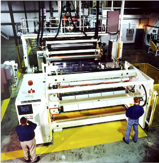
**Fig. 9-8** Cast film winder. Image provided by Davis-Standard
