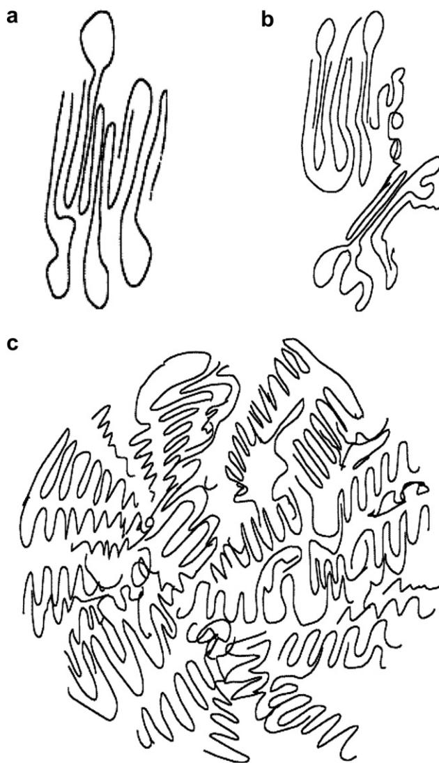
**Fig. 3-3** Semicrystalline structure of polypropylene. (a) crystallite formed from polymer chains associating; (b) secondary crystallization associating crystallites to form lamellae; (c) formation of spherulites from long range structuring of lamellae.
