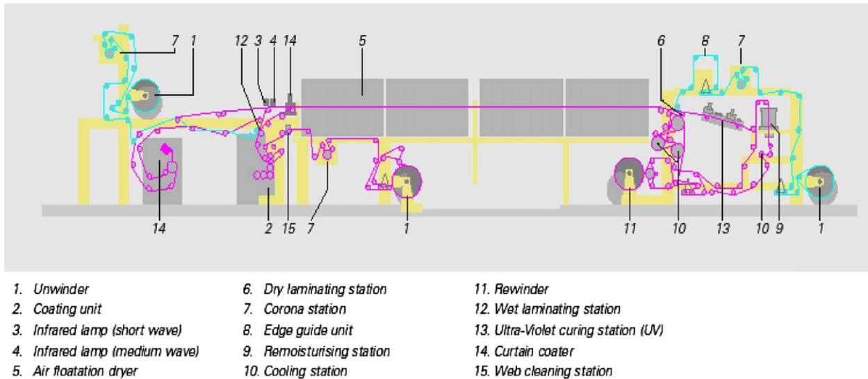
**Fig. 13-1** Coating machine with three unwinds and two laminating stations. Courtesy Polytype Converting SA.
