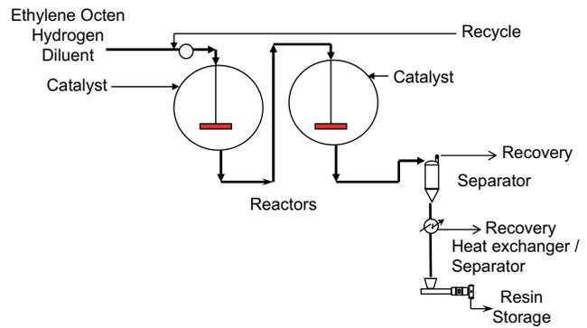
Fig. 2-26 Solution process (simplified).
