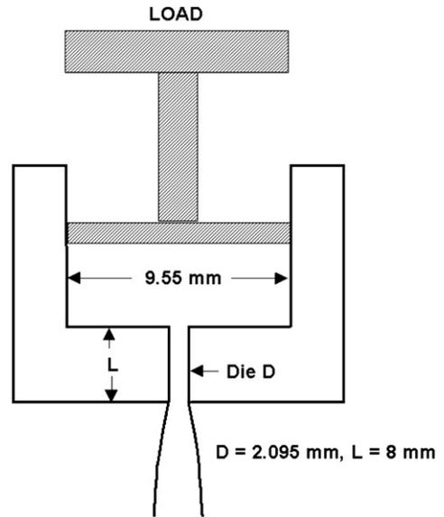
Fig. 2-3 Schematic of a melt indexer. ASTM D-1238 Under the conditions of the melt index measurement with the 2.16 kg load, the wall shear stress can be calculated to be  $\tau_w = 1.94 \times 10^4$  Pa ( $=2.814$  psi) and the wall shear rate approximately  $\dot{\gamma} = (1838/\rho)$  MI where  $\rho$  is the melt density. Assuming  $\rho = 766$  kg/m<sup>3</sup> for a typical PE melt at  $190^{\circ}\text{C}$ , we get  $\dot{\gamma} = 2.4 \times$  MI.
