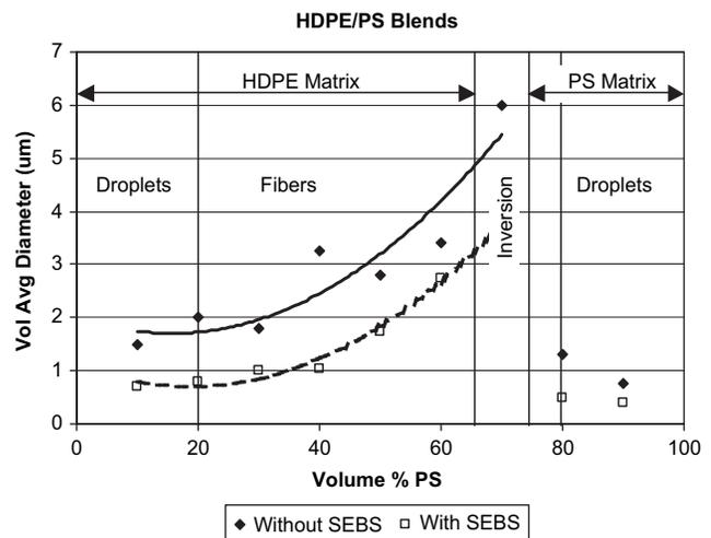
Fig. 12-20 Blend morphology as a function of concentration. PS-HDPE blends from Bourry and Favis [54].
