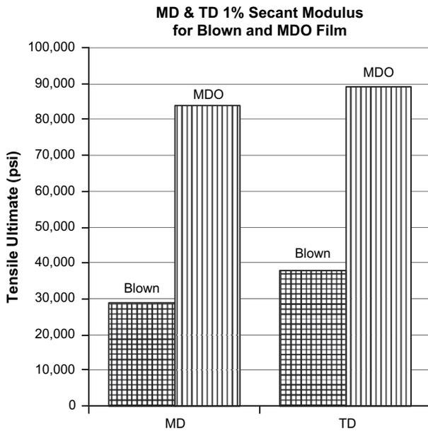
**Fig. 10-10** MD and TD 1% secant modulus for blown and MD oriented LLDPE [3].
