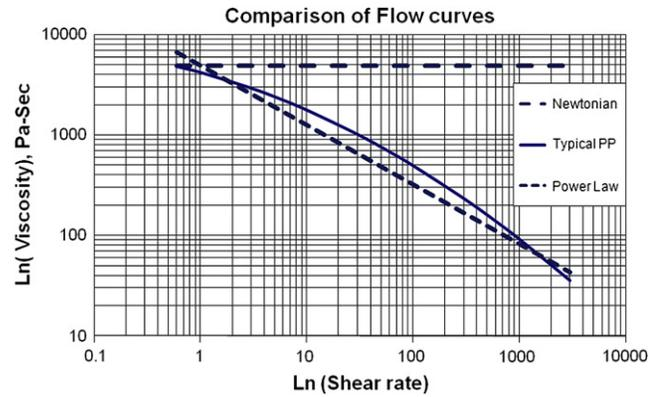
**Fig. 6-12** The viscosity versus shear rate for a Newtonian, a power law and a typical polypropylene (PP) melt.
