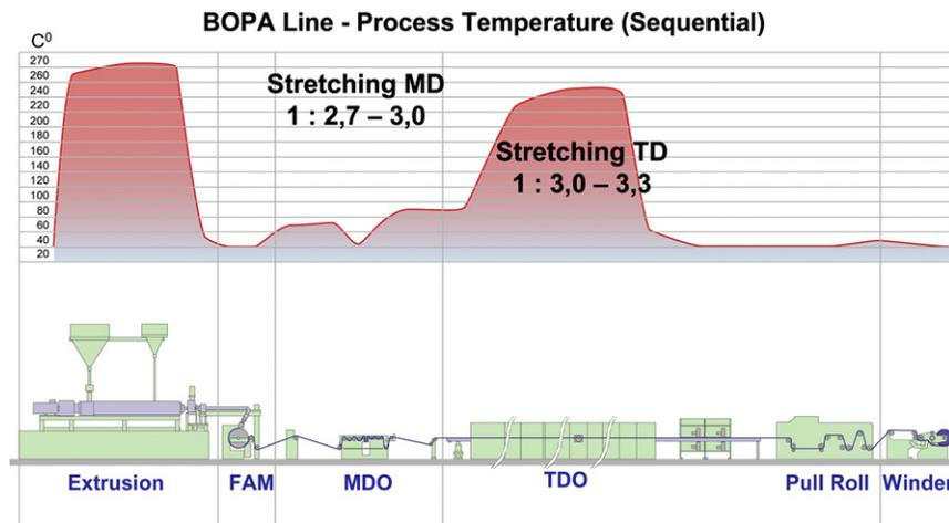
Fig. 11-26 Typical process conditions for MD/TD BOPA.
