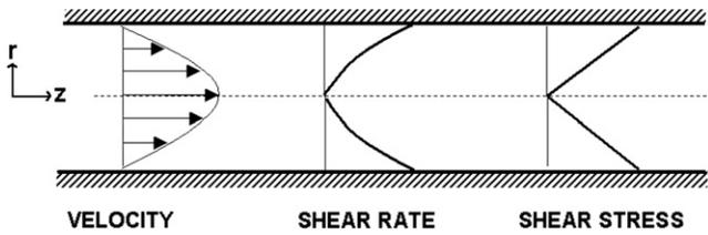
Fig. 5-5 Velocity, shear rate and shear stress profiles for pressure driven flow through a tube of radius  $R$ .
