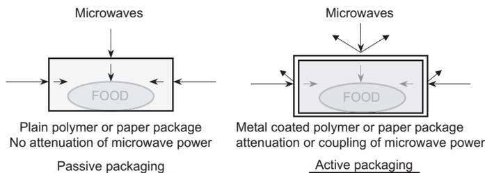
Fig. 14-5 A schematic comparing active and passive microwave packaging.
