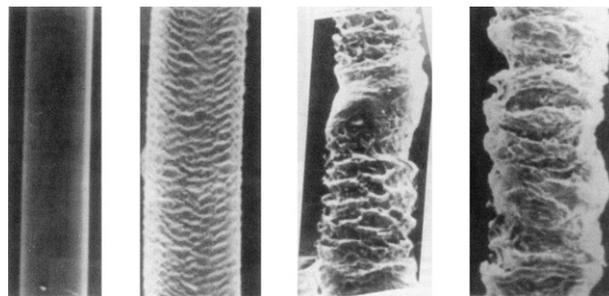
Fig. 5-14 LLDPE extrudates obtained from a capillary at apparent shear rates of 37, 112, 750 and 2250  $s^{-1}$ .
