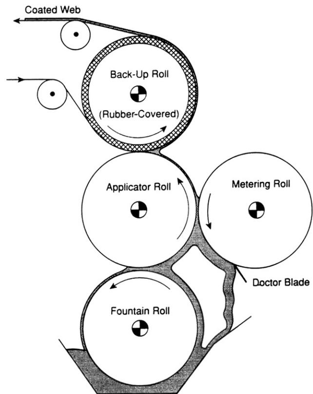
**Fig. 13-7** Four-roll pan-fed reverse roll coater. From *Modern Coating and Drying Technology*, (Cohen, E.D., Guttoff, E.B., eds), Copyright © 1992 Wiley-VCH. Reprinted with permission of John Wiley & Sons, Inc.
