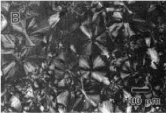
**Fig. 3-5** A Maltese cross pattern of birefringence obtained using optical microscopy under crossed polarizers. Polypropylene was isothermally crystallized at a pressure of 100 MPa.
