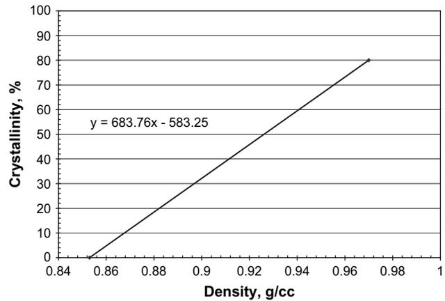
Fig. 2-7 PE polymer weight percent crystallinity as a function of density.
