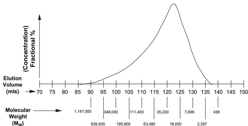
**Fig. 2-9** GPC curve showing concentration of various molecular weights of a polymer.
