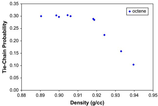
**Fig. 2-43** Probability of tie molecules in homogeneous octene copolymers as a function of density.
