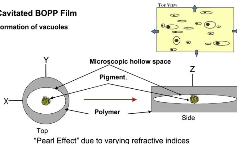
Fig. 11-17 Cavitated BOPP film mechanism.
