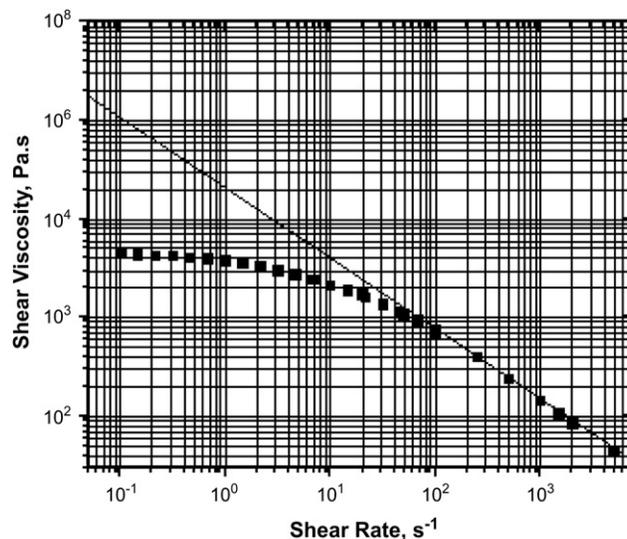
Fig. 5-3 Double logarithmic plot of shear viscosity versus shear rate. The straight line is the power law fit which fails at low shear rates. For this graph the coefficients for the straight line are:  $m \approx 20\,000 \text{ Pa}\cdot\text{s}^n$ ;  $n \approx 0.3$ .
