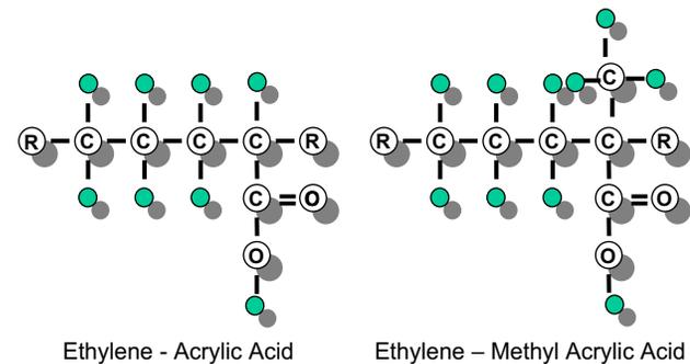
Fig. 2-21 Acid copolymers of ethylene.
