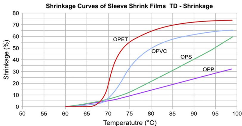
Fig. 11-34 TD shrinkage versus temperature for four shrink films.
