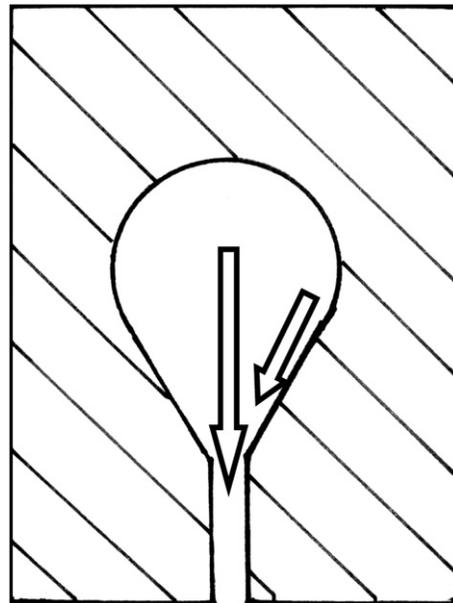
**Fig. 6-23** Streamlined manifold design eliminating sharp transition from manifold to land as in Fig. 6-21
