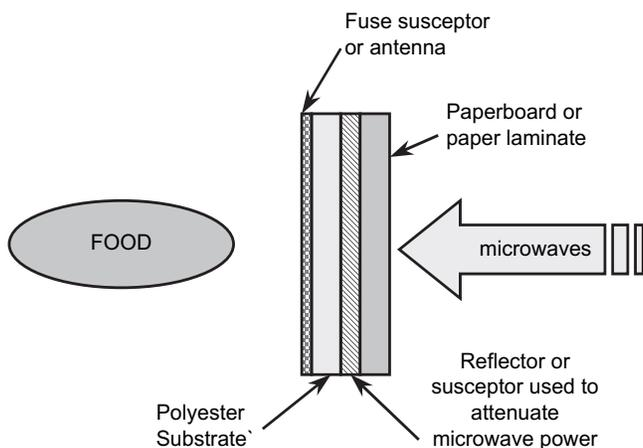
Fig. 14-6 A simple packaging structure.
