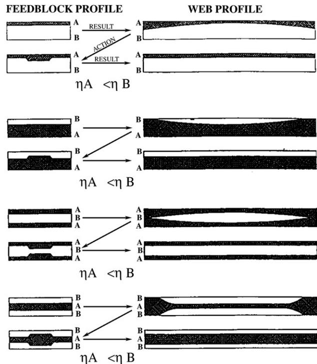
Fig. 5-16 Feedblock profiling and the resultant effects.
