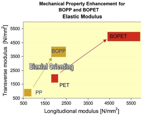
**Fig. 11-3** Mechanical property enhancement for BOPP and BOPET.
