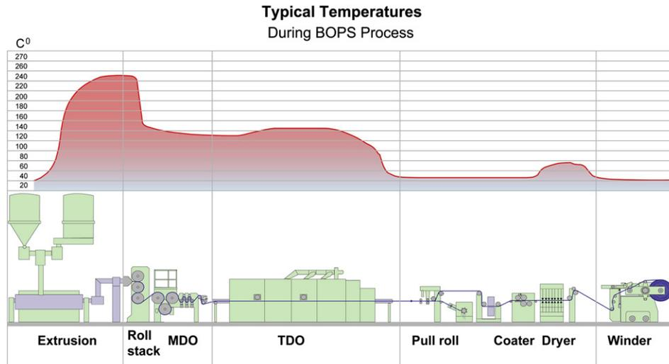
Fig. 11-30 Typical BOPS process temperatures.
