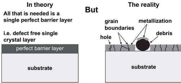
**Fig. 14-17** A schematic comparing a theoretical and a real barrier coating.
