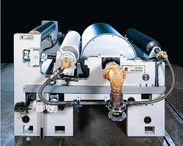
**Fig. 9-11** Extrusion coating/laminating station. Image provided by Davis-Standard <http://www.davis-standard.com/>.
