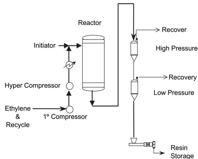
**Fig. 2-14** Autoclave reactor (simplified).
