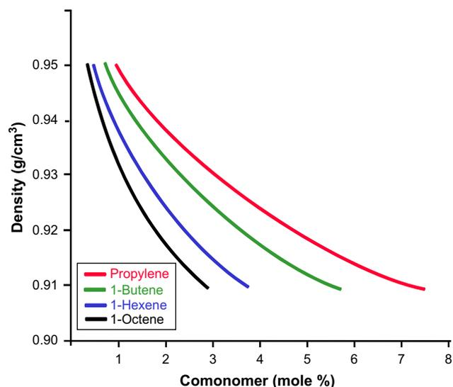
**Fig. 2-36** Comonomer versus density for various alpha olefins.
