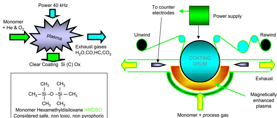
Fig. 14-16 A schematic of the PECVD process using hexamethyldisiloxane (HMDSO) as the precursor.
