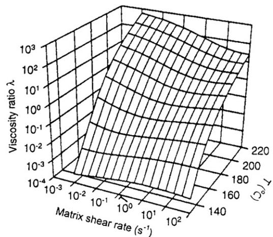
Fig. 12-22 HDPE-PS blend viscosity ratio variation as a function of shear rate and temperature. Taken from Huneault et al [80]. Courtesy of the Society of Plastics Engineers.
