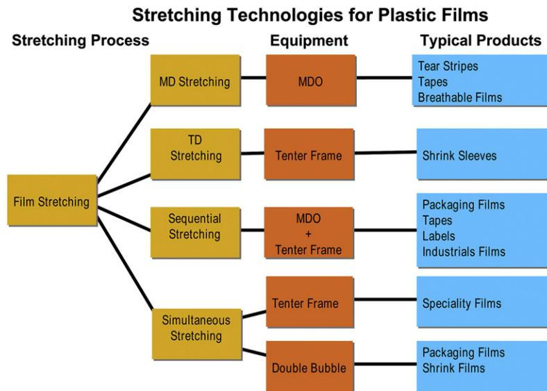
**Fig. 11-4** Plastic film stretching.
