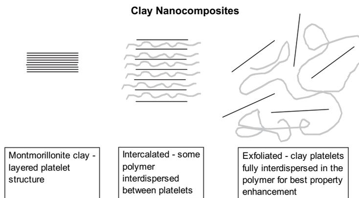
**Fig. 12-27** Illustration of states of clay nanocomposites.
