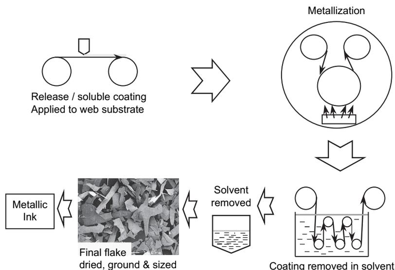
**Fig. 14-4** A schematic of the flake metallic pigment production process.
