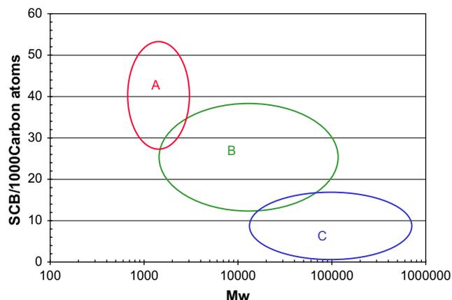
Fig. 2-31 Branching distribution and  $M_w$  of a multiple site Z–N supported catalyst producing a heterogeneous polymer.
