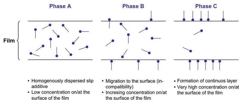
Fig. 4-6 Principal mode of action of slip additives.
