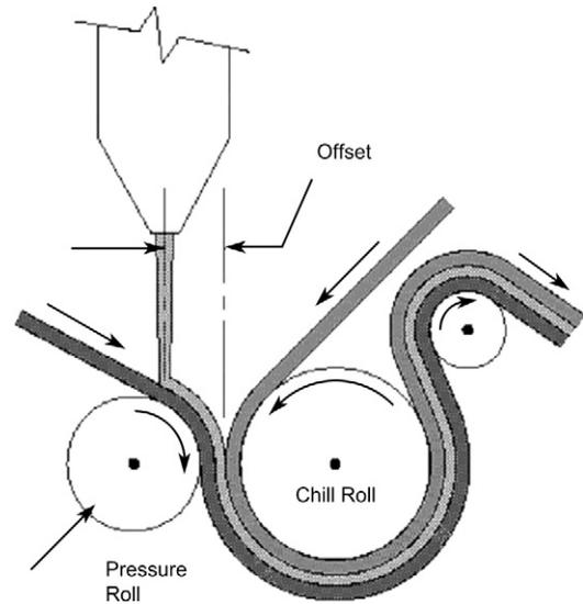
**Fig. 9-9** Extrusion lamination detail.
