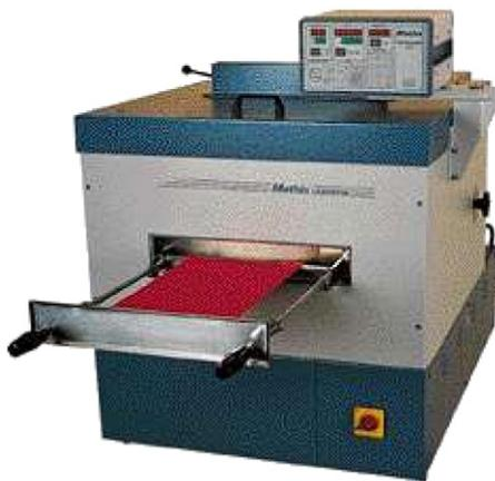
**Fig. 13-3** Laboratory sheet coater. Courtesy Werner Mathis USA.
