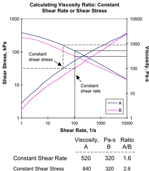
Fig. 12-21 Calculating viscosity ratio.
