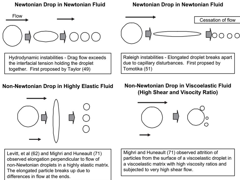
Fig. 12-18 Single droplet break-up mechanisms in shear flow.
