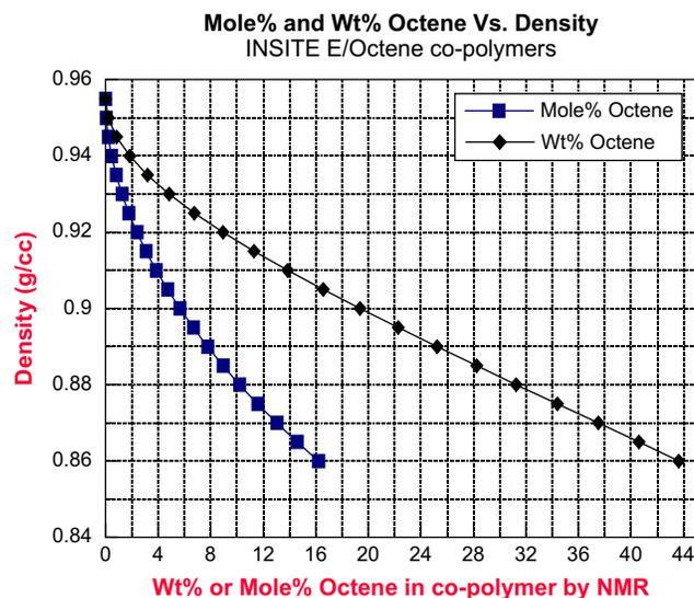
Fig. 2-6 Density as a function of comonomer level.
