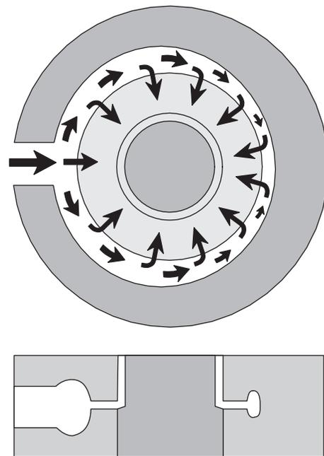
**Fig. 7-5** A typical side-feed distribution system.
