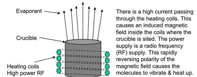
Fig. 14-13 A schematic of an induction heated evaporation source.
