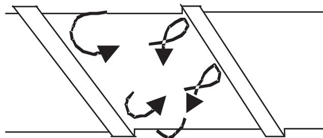
Fig. 12-3 Illustration of circulatory flow patterns in the metering section of a single-screw extruder. Adapted from Middleman [21].
