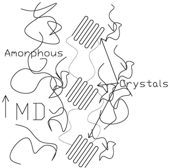
**Fig. 10-2** Crystal and amorphous arrangement before orientation.
