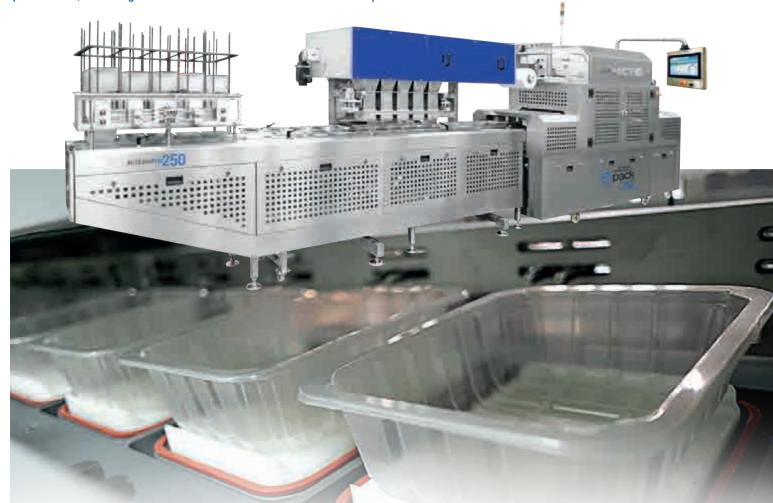
The autoMAP-MD250 is a high-speed, fully automatic MAP packaging machine that can meet the demands of high-capacity mass production. The machine can perform all stages of the packaging process, from tray feeding, weighing, sorting, MAP sealing, labeling, collecting, and stacking the product. The PLC automation unit monitors and controls all aspects of the production line, providing real-time warnings for possible errors, misuse, or installation malfunctions and protecting the system.
