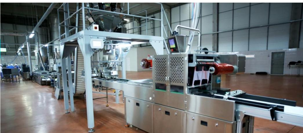
Our **autoMAP 100-200** serie full automatic packaging line machines provides quick service and cleaning facilities by easy-removable side covers . All frames and intermediate elements were manufactured with ISI304 stainless steel.
