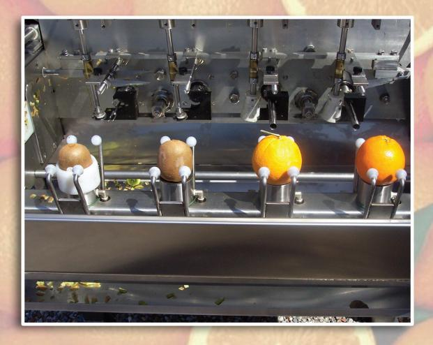
The semiautomatic peeling machine for oranges and kiwis at manual load can be at 2 or 4 processing stations.
