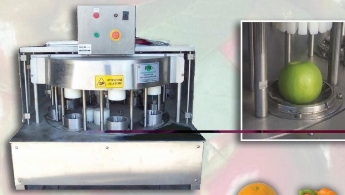
The machine has a structure in stainless steel and food-approved material. All components are easily interchangeable, because they are produced to one design on NC-machine. All parts in touch with the fruit are suitable for hygienic and alimentary purposes. Besides, the interior parts of the machine are protected by carters in stainless steel to avoid accidents to the workers who use the machine. Changing the blades it is possible having fruits in different forms and sizes.
